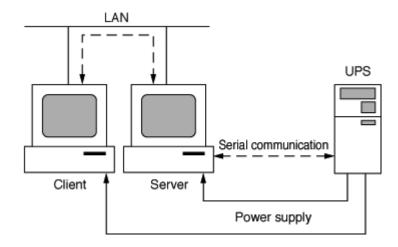
Fig.7 Configuration example using SNMP card
